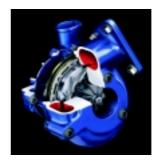
VNT turbochargers adjust the gas cross section at the inlet of the turbine wheel in order to optimize turbine power with the required load. At low engine speed and small gas flow, VNT turbochargers reduce the cross section, increasing
